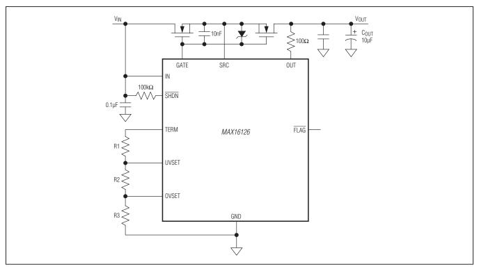
Figure 5. MAX16126 Typical Operating Circuit
