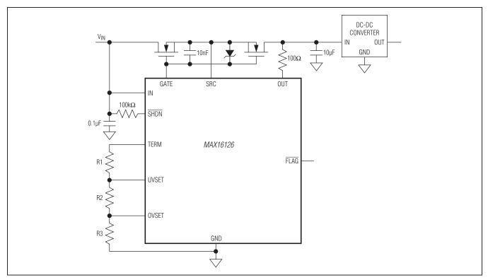
Figure 1. Overvoltage and Undervoltage Window Detector Circuit (MAX16126)
