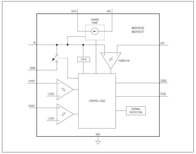
Figure 7. MAX16126/MAX16127 Functional Diagram
