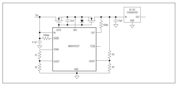
Figure 2. Overvoltage and Undervoltage Limiter Protection Configuration (MAX16127)
