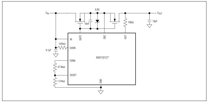
Figure 4. Use of a 6.8V Zener Clamp to Enable Operation with  $V_{\rm IN}$  Up to 35V
