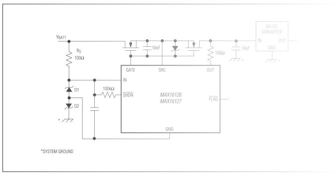
Figure 3. Circuit to Increase Input Voltage Protection Range
