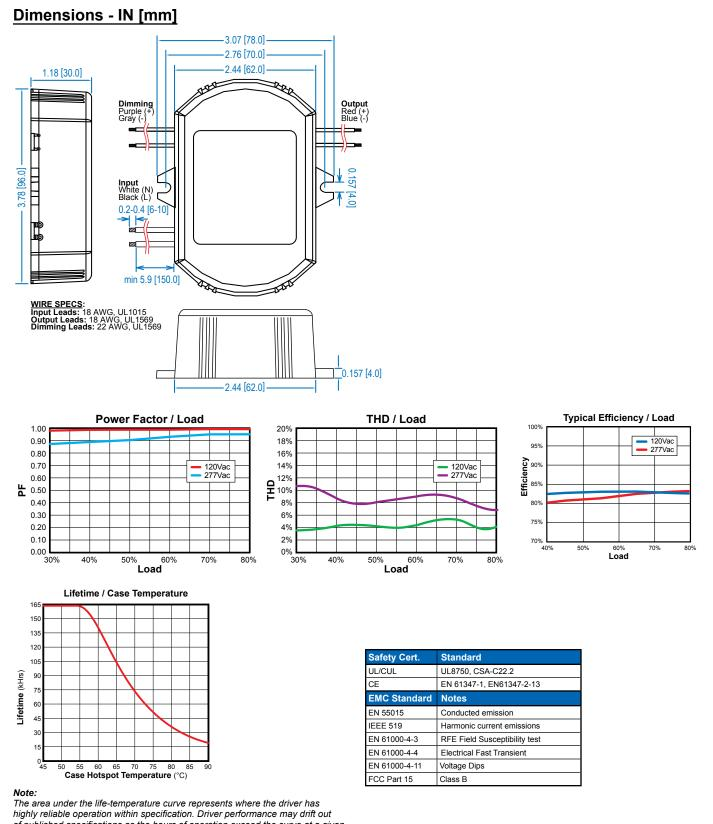
The area under the life-temperature curve represents where the driver has highly reliable operation within specification. Driver performance may drift out of published specifications as the hours of operation exceed the curve at a given temperature. Higher operating temperatures increase the chances of a failure to function. Other electrical, mechanical and environmental factors affect driver lifetime but are not represented in this calculation.
