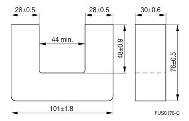
U cores are supplied as single units. The  $A_L$  value in the table applies to a core set comprising two ungapped cores.
