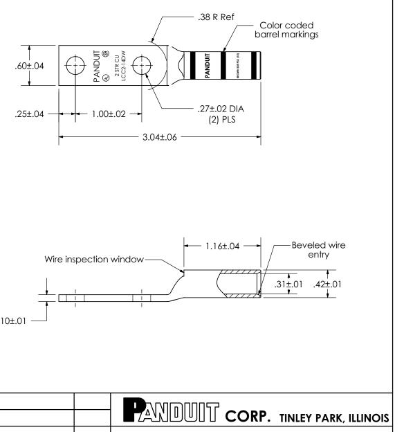
LCC2-14DW-Q Copper Lug - Two-Hole, Long Barrel with Window
